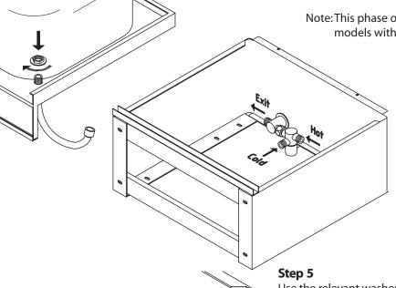
Use the relevant washer and the grooved nut to fix the mixer tap on the frame, lining the small screw in the mixer tap up with the hole in the washer (as shown in the diagram)
