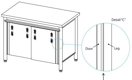
1) To adjust sliding doors it's necessary loosen the screws TBC M6x14 that support the same doors (look at details "A" and "B"). Then, proceed with adjustment of the door, raising it or lowering it, so that it is in parallel with the leq (look at detail "C"), or, in case of module structure, in parallel with the side of structure (look at detail "D").
