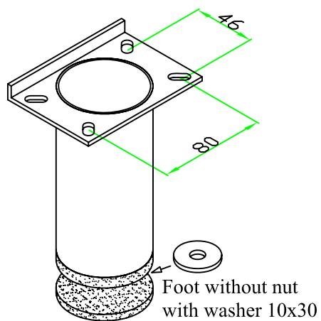
**BendoniInox** Tube Ø60,3 - Cupboard sliding doors lateral type plate (0104)
