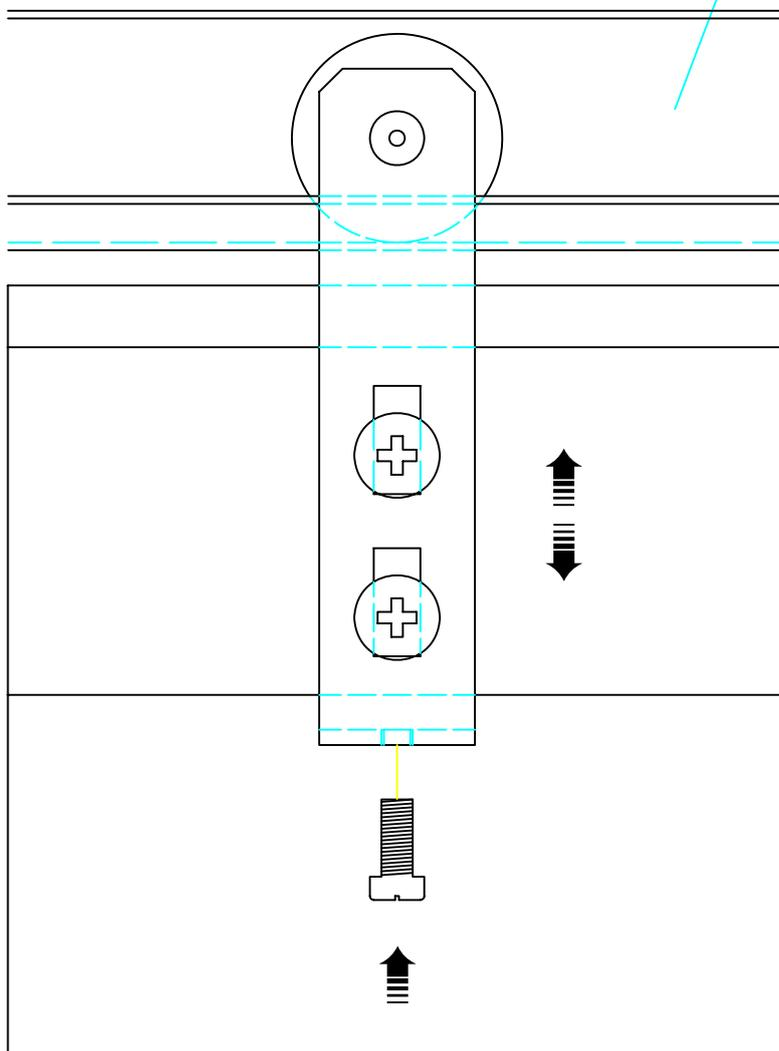
Air between door and guide can oscillate from a minimum of 1 mm and a maximum of 3 mm
