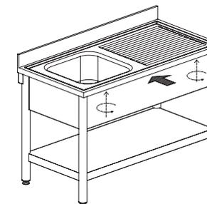
7) Push the Top towards the side of the wall by roughly two cm and apply the two screws M4x16 under the front edge.
