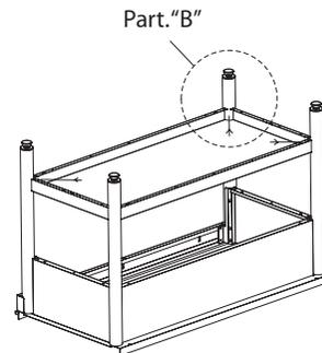
4) Depending on the sink is on legs or have lower shelf apply the rear connecting cross member or the lower shelf using supplied screws (as upper drawings). Check that all the screws are screwed and tighten.
