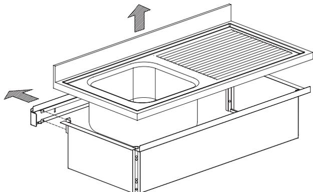
3) Place the structure upside down (as drawing) and apply the legs at the structure using supplied screws M10x40. Don't tighten the screws!! At this point apply rear band (previously removed) using the four cross head M6x25 screws. Don't tighten the screws!!
