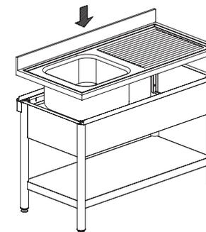
6) Replace the Top on the structure placing it at a right angle (as upper drawing).
