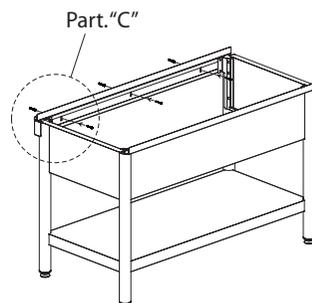
5) To avoid accidental movement of the sink after installation we recommends the fixing to wall using the proper holes in the rear band and the anchor bolts supplied together with set of sink accessories (see Part. "C").
