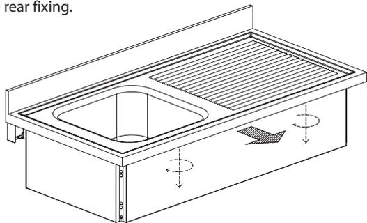
2) Once it is free from rear fixing and from the front edge remove the Top, lifting it at a right angle. Remove the rear band, pre-assembled from us, unscrewing the four cross head M6x25 screws.
