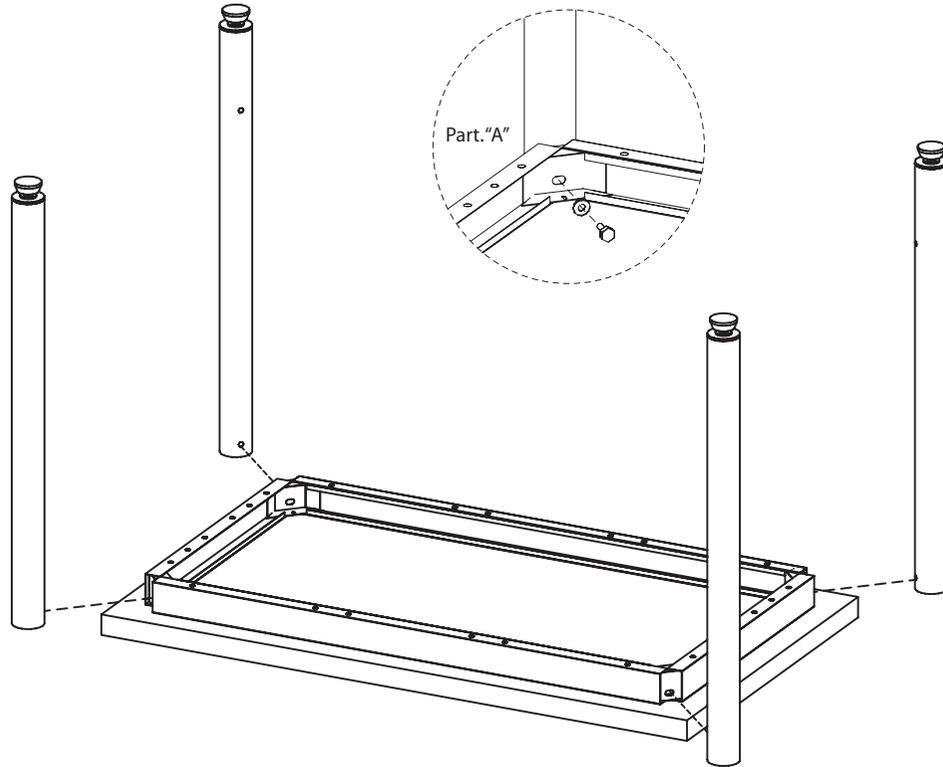
2) Apply the legs at upper band of the table (supplied already fixed on the working Top) using the 4 screws TE 10x20 together with the washers supplied, without tighten them.
